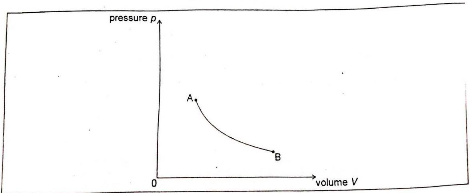
Process AB is an isothermal change, as shown on the pressure volume ( $pV$ ) diagram, in which the gas expands to three times its initial volume.
