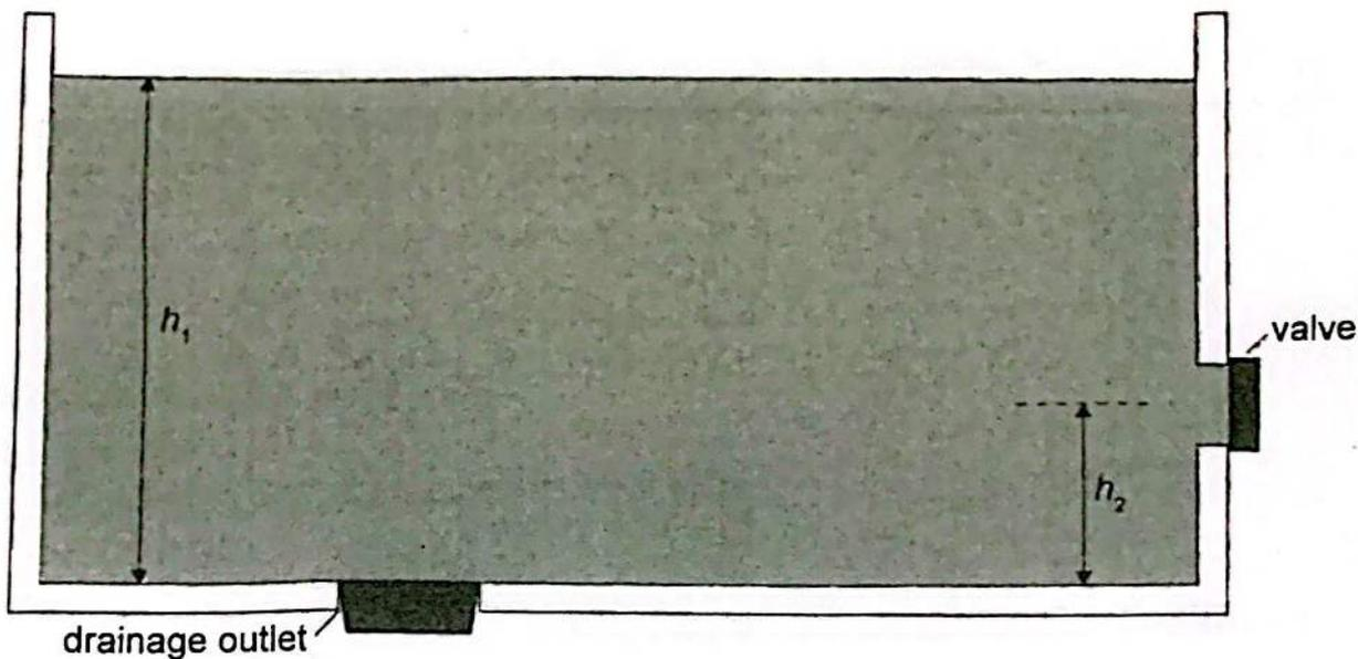
The drainage outlet has a diameter of 100 mm and a metal stopper of mass 2.5 kg is used to plug the outlet.
